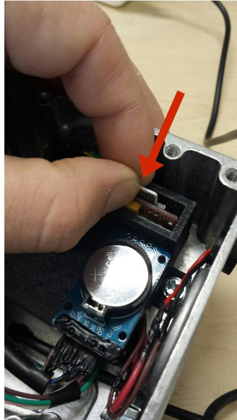
APÓS INSERIDO NO LOCAL ADEQUADO, EMPURRE O CHIP ATÉ O FIM DO SLOT COM CUIDADO ATÉ SENTIR UM "CLICK" INDICANDO QUE ELE ESTÁ SEGURO NO LOCAL, CONFORME A PRÓXIMA FIGURA:
